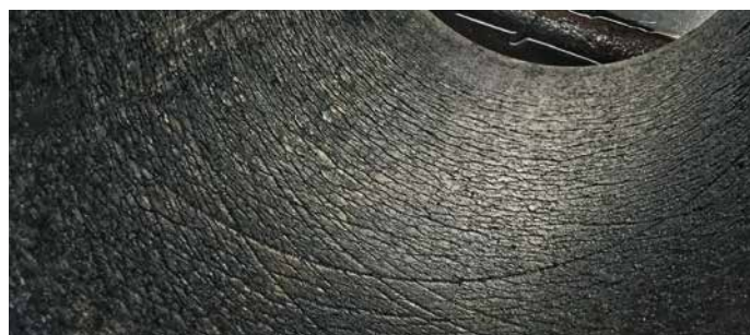
SA718 (1250 – 1400 MPa) after 150,000 Cu billets, fine network of cracks
