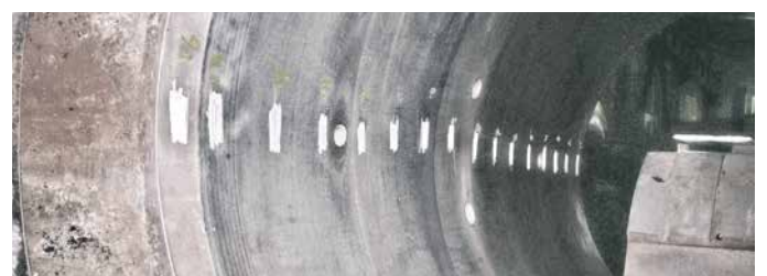
Hardness test on container ▲
