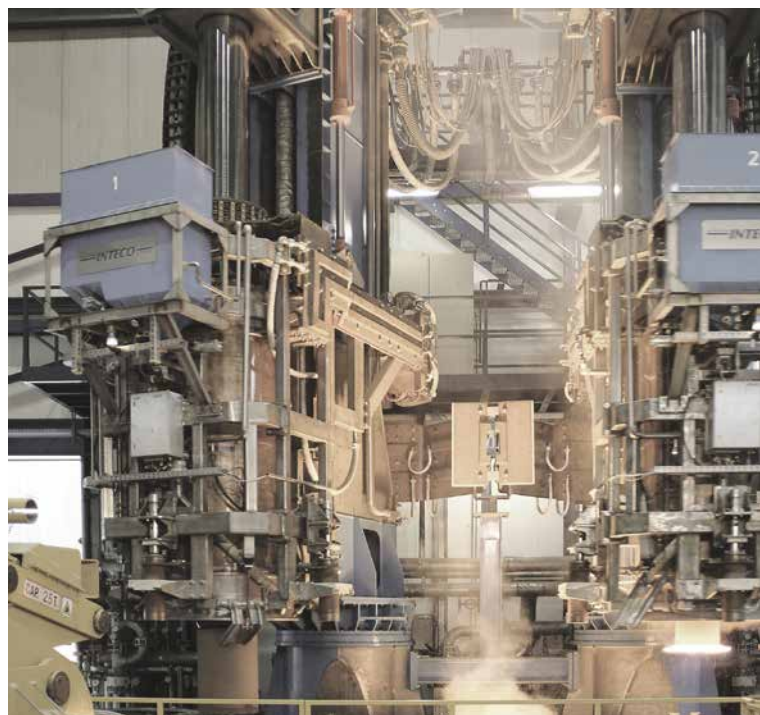
Electro-slag remelting process (ESR) ▼
