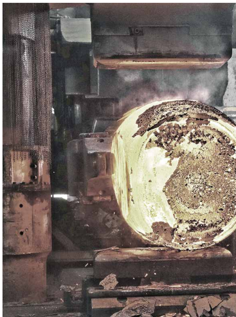
Forging of ESR ingot on the 30MN-press ▲
