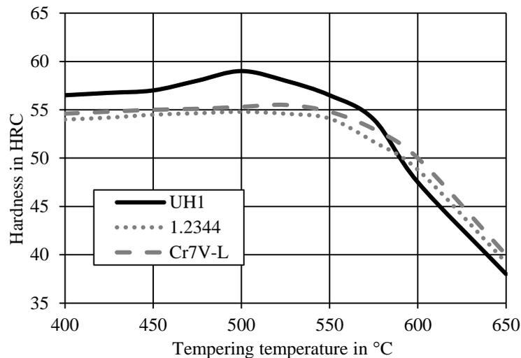
Fig. 1. Tempering curves of the three steel grades
