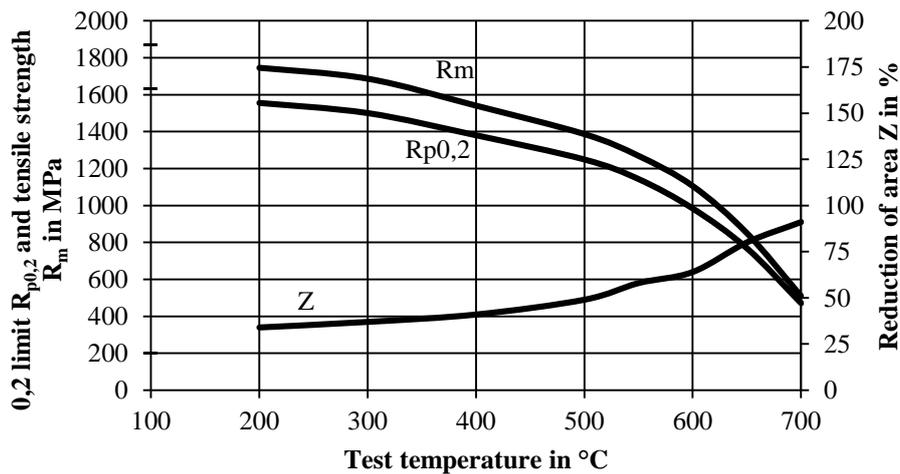
Fig. 3. High-temperature strength graph of premium tool steel UH1
