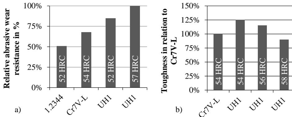
Fig. 2. Schematic comparison of abrasive wear resistance (a) and toughness (b)
