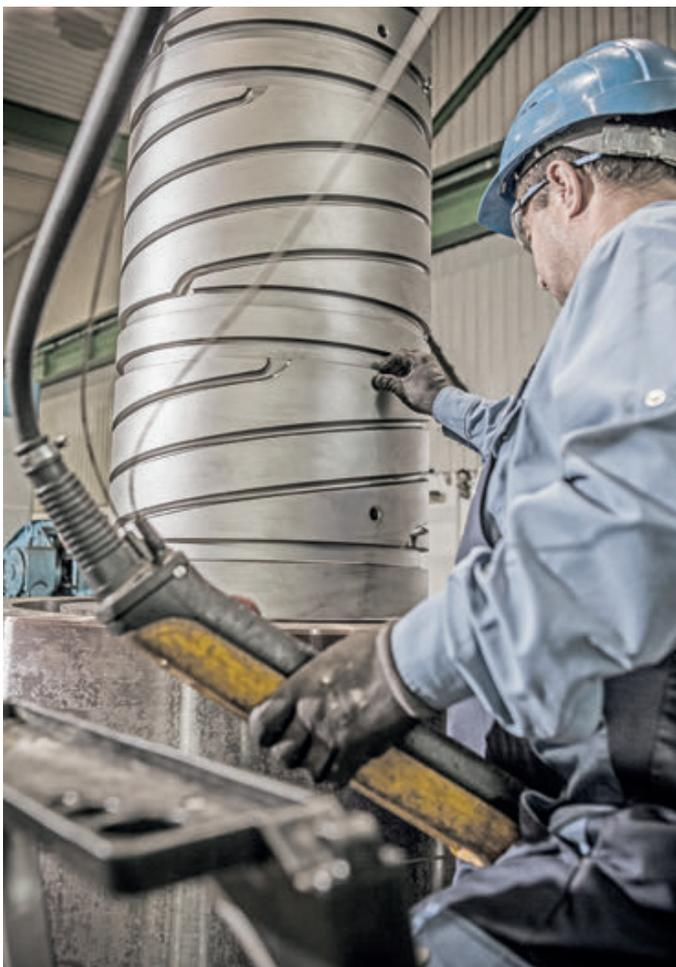
construction design for direct presses are quite different from those for the construction of containers for indirect extrusion. The specialty of KSAI is to offer a choice of steels for the liners and all the parts that make up the containers and the tooling in steel for the presses, from casting, forging to machining and heat treatment”.
