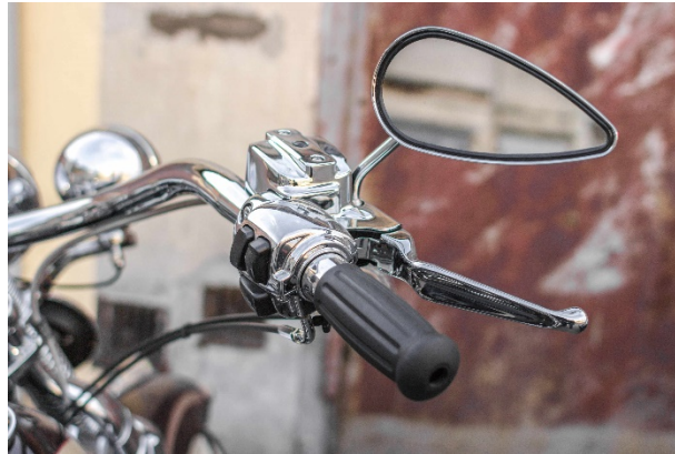
Figure 8- Die cast and chromium-plated brake fluid tank of a motorcycle (example).
