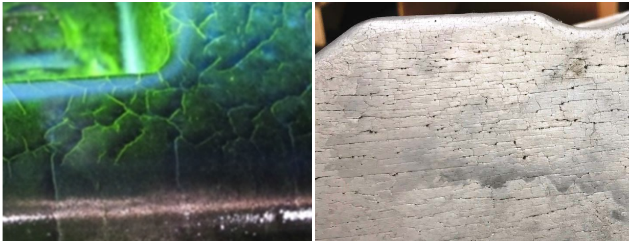
Figure 2- Thermal shock cracks on the surface reduce the quality of the cast product. Typical crack appearance under UV-light during magnetic particle test (left); Traces of severe thermal shock cracks on the surface of a cast product (right)
