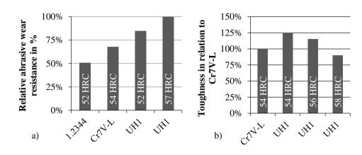
Fig. 2. Schematic comparison of abrasive wear resistance (a) and toughness (b)
