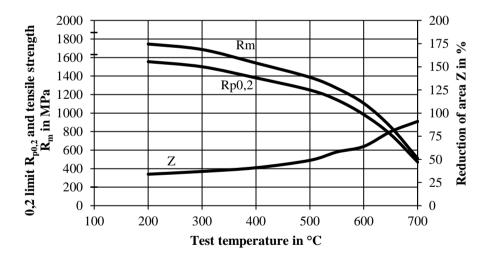
Fig. 3. High-temperature strength graph of premium tool steel UH1
