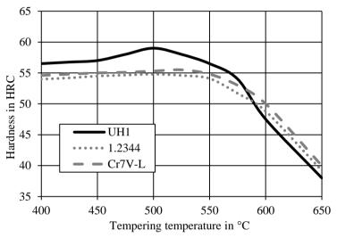
Fig. 1. Tempering curves of the three steel grades
