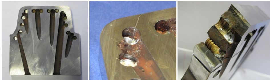
Fig. 7. Section through a defect hot-stamping tool Left: Cross-section; Middle: Detail with crack from cooling channel to the working surface; Right: Corroded crack surfaces
