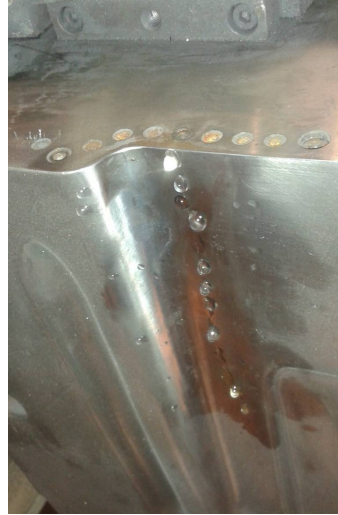
Fig. 6. Water leaking from a cooling channel in a hot-stamping tool.
