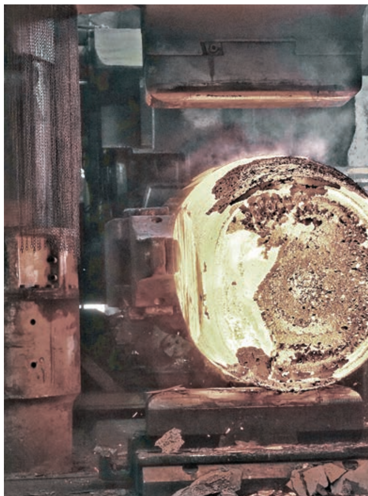
Forging of ESR ingot on the 30MN-press ▲
