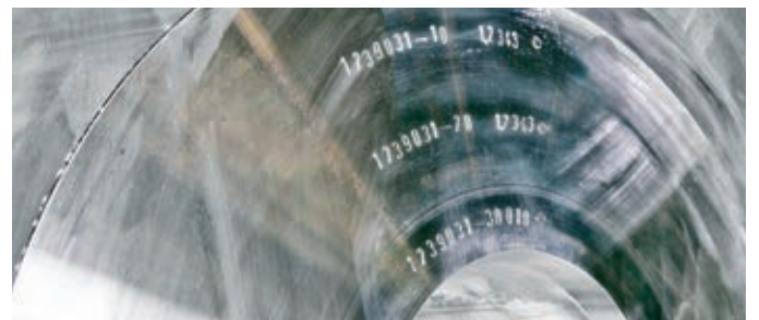
▲ Container for aluminium extrusion with Q10 inner sleeve
