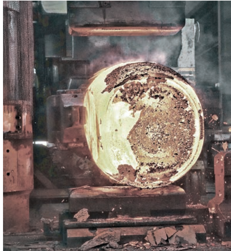
Forging of ESR blocks on the 30MN press ▲
