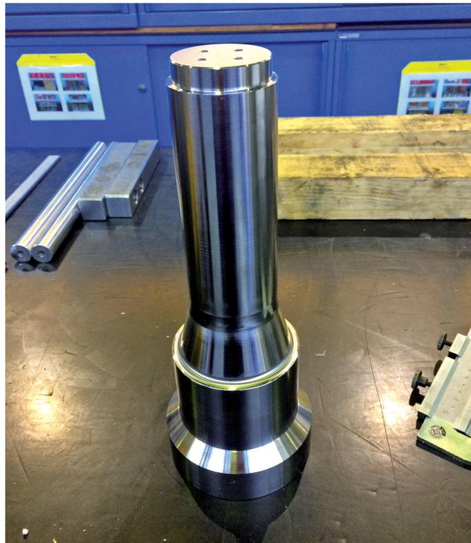
Extrusion punch of CS1 (55-57 HRC)
