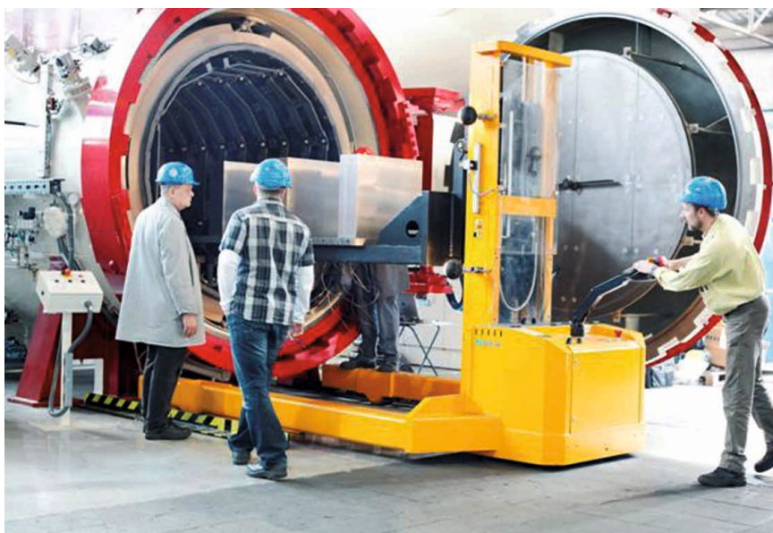
Figure 4: Modern vacuum hardening furnace at Kind & Co. for pressure die casting dies weighing up to 6,000 kg (Photo: Georg Fischer AG)
