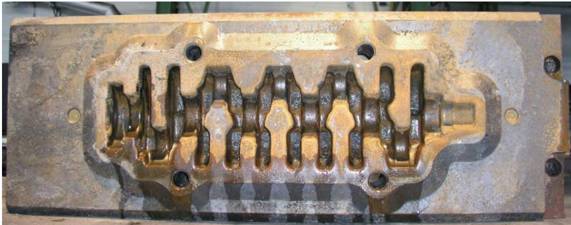
Figure 8: Crankshaft forging die made of CR7V-L with a hardness of 45 HRC achieving a performance increase of 60 % compared to 1.2343 respectively 1.2344.
