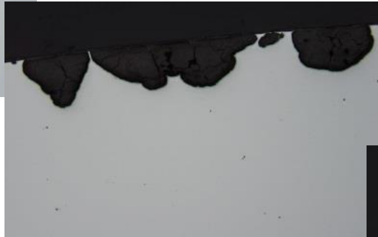
Localized corrosion Mostly at local inhomogenities or non-metallic inclusions
