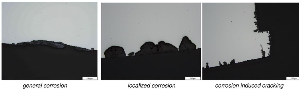
**Figure 5:** Microscopic appearance of different corrosion defects
