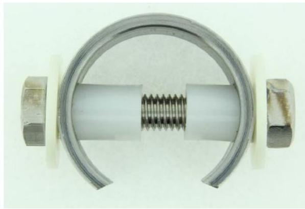
**Figure 3:** Sample for corrosion tests (photo courtesy of WITg)
