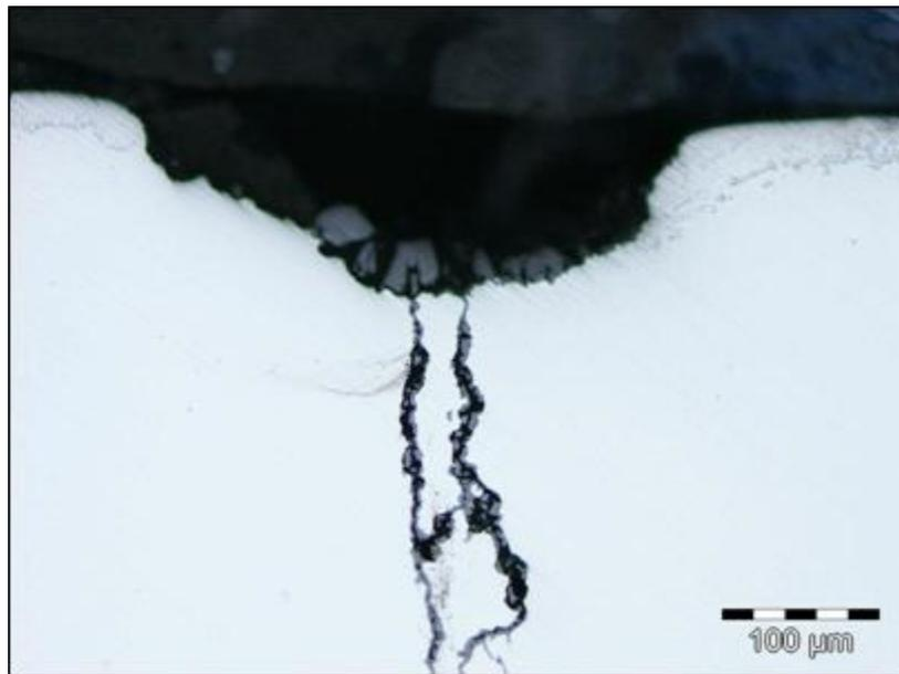
**Figure 6:** Corrosion induced stress cracks propagating from corrosion pits in cooling channels to the tool surface
