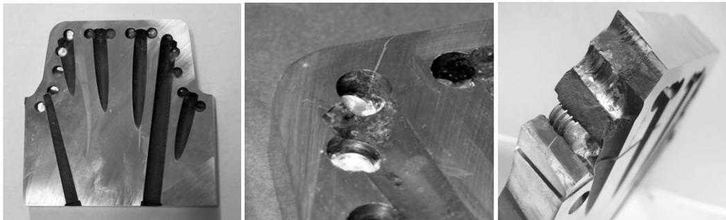
**Figure 1:** Corrosion induced crack from a cooling channel to the working surface of a hot-stamping tool
